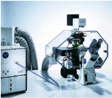
Fig. 49: A climate chamber offers features like control of temperature, humidity and CO 2 content of the atmosphere.
