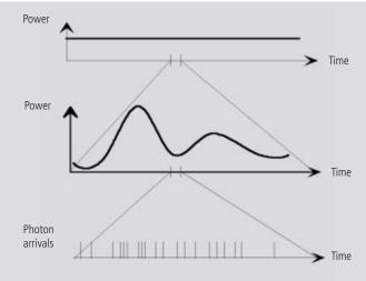
A resolution probability of 90% is considered necessary for resolving the two point images. Accordingly, the two-point object defined above can only be resolved if each point produces at least about 25 photoelectrons. With pinhole diameters smaller than 0.25 AU, the drastic increase in shot noise (decreasing intensity of the detected light) will in any case lead to a manifest drop in resolution probability, down to the level of indeterminateness ( $\leq$  50% probability) at PH = 0.
