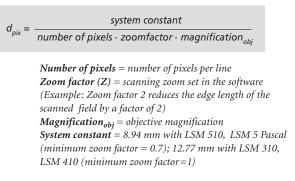
The minimum scanning zoom needed to fullfill the Nyquist theorem can therefore be calculated as follows:
