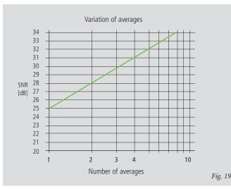
Figures 18 and 19 Improvement of the signalto-noise ratio. In figure 18 (top), pixel time is varied, while the number of signal acquisitions (scans averaged) is constant.
